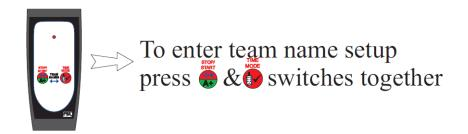
To change the letter to be adjusted press the appropriate button on the transmitter to move the flashing underscore to the right or left e.g. "T\_{"}" to "TE\_" There are separate buttons for the home & away teams
