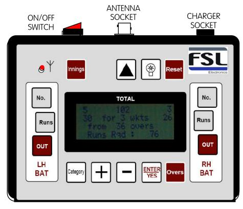
The console is powered by an integral rechargeable battery pack and the charger supplied plugs in to the socket at the rear of the console. The charging and operating time will vary depending on use, but typically an overnight charge will power the console for around 8 hours. Should the batteries go flat during use, simply connect the charger and continue to use whilst charging. On models fitted with a backlit display, this will illuminate when the charger is connected.
