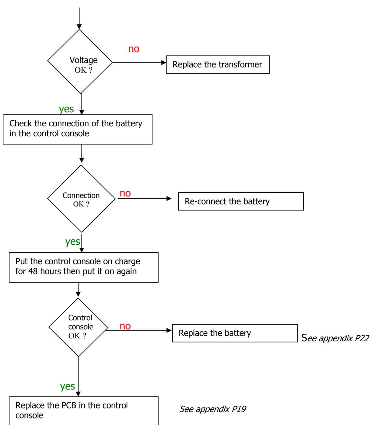
**PROBLEM No2 :** The control console displays a line on top of the LCD
