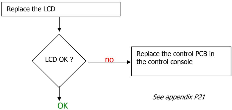
**Problem No3 :** The datas are displayed on the LCD but the keys of the control console do not work
