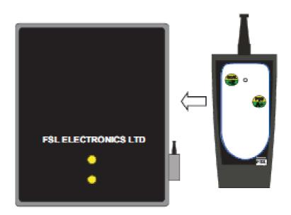
To blank the scoreboard display, press the & The score will be restored if any score button is pressed
